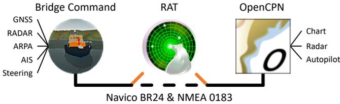
Fig. 5. The radar simulation environment consists of two components. Bridge Command (BC) simulates a virtual ship and surrounding vessels, while OpenCPN serves as a chart plotter, including a radar display and an autopilot. Finally, RAT (Sec. VI) injects radar cyberattacks into the network traffic.
