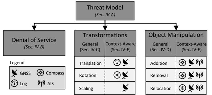
Fig. 3. Network-based attacks on marine radar systems can be classified into *Denial of Service*, *Transformation*, and *Object Manipulation*. By incorporating external situational knowledge (indicated by respective icons), these basic types can be enhanced to stealthier *context-aware* attacks.
