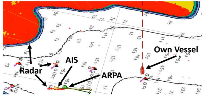
Fig. 2. Radar visualizes landmasses, buoys, and surrounding vessels (red). Moving targets can be tracked with ARPA (green circles), which are additionally complemented by AIS broadcasts (yellow triangles).
